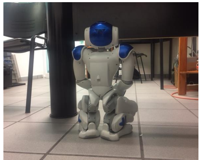
Figure 1 This image shows a case where the NAO robot needs to move to the other side of the desktop. However it is obstructed by a chair, so it is not possible to move, the only possibility to move is four legs under the desk or chair.
